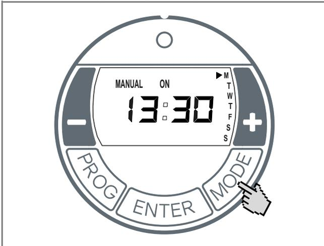
Pressing the MODE key switches the operating mode between MANUAL ON, MANUAL OFF and AUTO.
